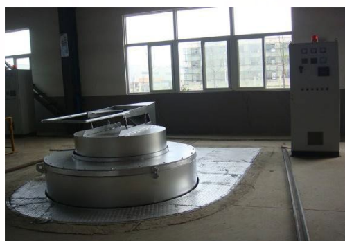
热处理炉 Heat Treatment Furnace
